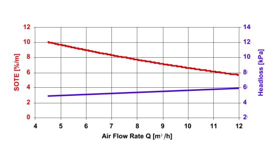
Oxygen transfer efficiency and headloss Tube Diffuser TD 63/2100, low plasticiser membrane
